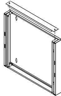
【3】 Fix the top and bottom of the back frame by 4 pcs of M5\*10 Self-tapping screw.
