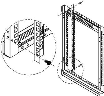
【4】 Fix 19" mounting rails to the first holes of top & bottom of side frames by 4sets of M5 screws.
