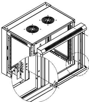
【7】 Install front frame by 4pcs of M6\*12 screws (6pcs of M6\*12 screws if more than 18U), refer to the picture.
