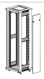
[ 9 ] : install side panels. adjust the diagonal dimension of cabinets.
