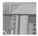
[7]: Install front door, rear door. Put the door block to the hole of the bottom of frame, and set the front door/rear door. Fix the top of front/rear door by bolts and top of frame.
