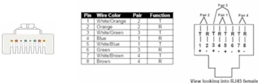
Figure 5. CAT5/5E/6 Straight Through UTP/STP Cable (8P8C)
